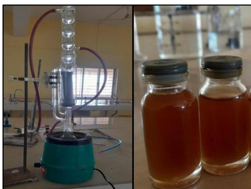
Figure 2. Soxhlet extraction of Linseed oil
