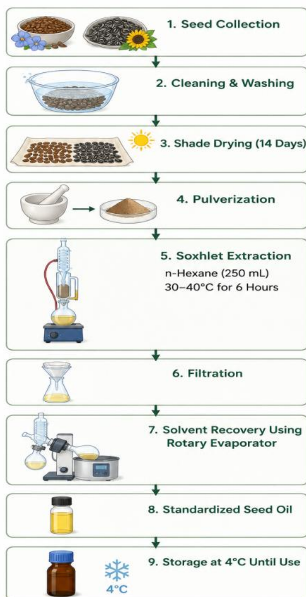
Figure 1. Flow diagram for extraction of seed oils
