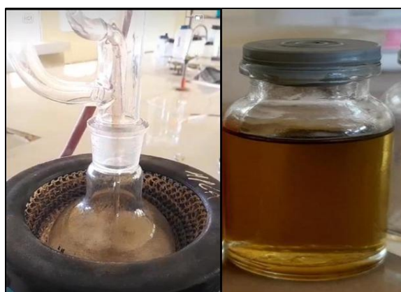
Figure 3. Soxhlet extraction of Sunflower oil
